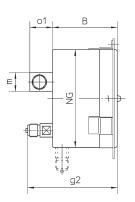
Mounting brackets welded to the case, and a separate front flange
